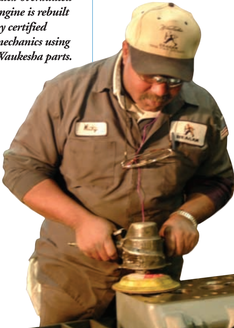
Many distributors have invested in special tools such as this head builder.
