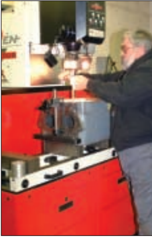
Many distributors have invested in special tools such as this head builder.
