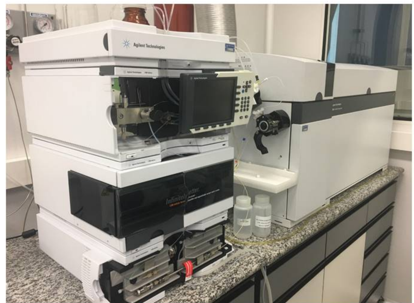
Figure 6. High performance liquid chromatography (HPLC) connected to Agilent 8800 Triple Quadrupole for Mercury Speciation. Phenomenex Sinergy Hydro-RP (C-18) 150 x 4,6 mm, 4 µm) Column was used.
