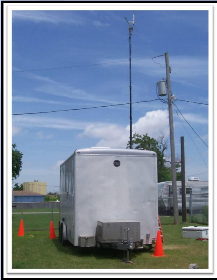
R5 Mobile Monitoring Trailer - note mast and inlet
