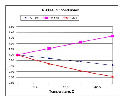
Data presented by Bullock /Bul99/ and Ward /Wel99/ show similar reductions in performance at high ambient temperatures. Bullock also reported that system design factors (coil face velocity and internal volume) can improve the performance of R-410A systems at high ambient temperatures. Therefore, variations in the high ambient performance can be expected between different product designs.
