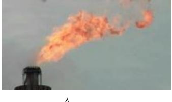
Good Combustion: Turbulent, Hot Flame Excess Steam/Air: Dilution and Cooling of Flame
